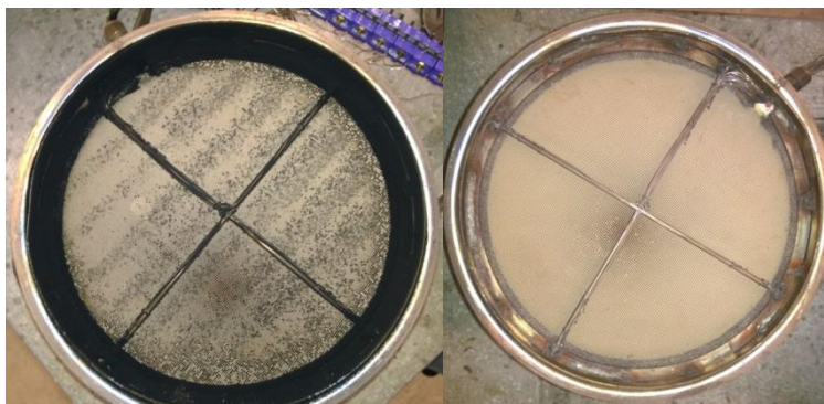
Figure 3.11. Comparison between the Physical Condition of the DOC Pre (left) and Post (right) a Thermal Aging Routine.
