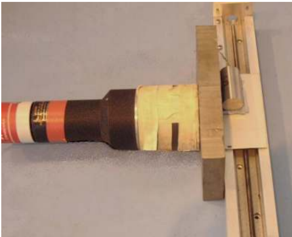
Figure 14: Photograph of the machine slide experiment used for powder distribution and fill-height measurements of the AE4043/n sources.
