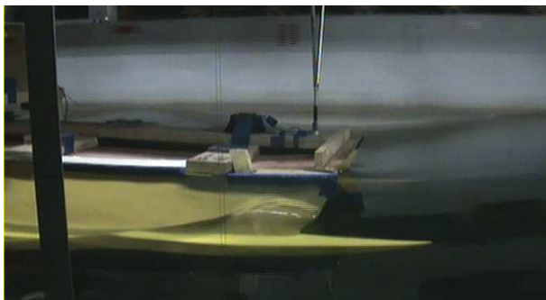
Figure 3c.: Seakeeping test in following waves conducted in towing tank of University Teknologi Malaysia (UTM).
