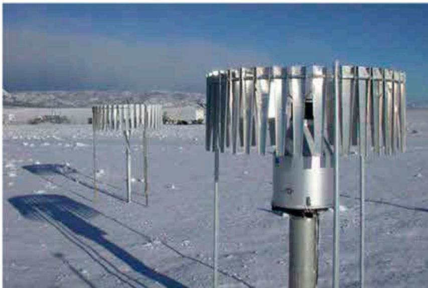
FIG. 1. An SA-shielded Geonor 600-mm gauge installed at the Marshall Field Test Site in Boulder.
