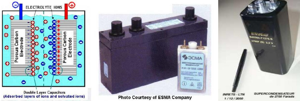
FIG.IV-18 – COUPE SCHÉMATIQUE ET VUE DE SUPER-CONDENSATEURS [ST-CEA]
