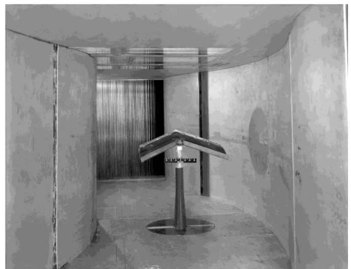
Figure 5. A view inside the Langley Stability Tunnel curved test section [16].
