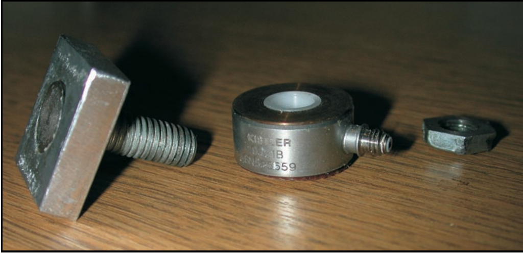
Figure 3.9: Load cell and sample holder.
