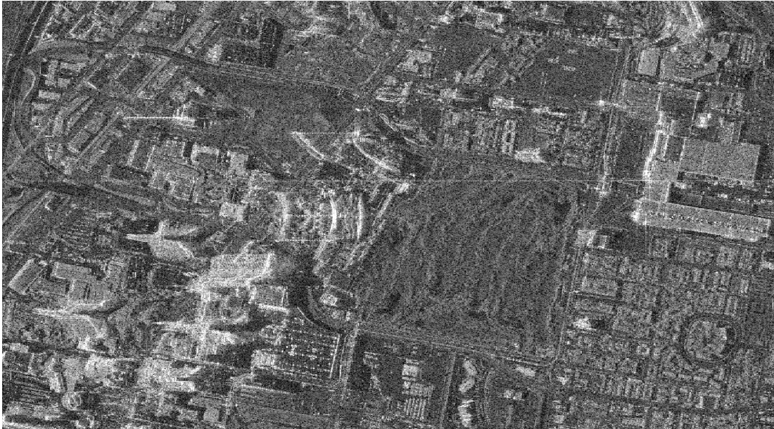
Figure 1.1 TerraSAR-X amplitude image at las Vegas, USA. Resolution: 1.1m*0.6m (azimuth and range)
