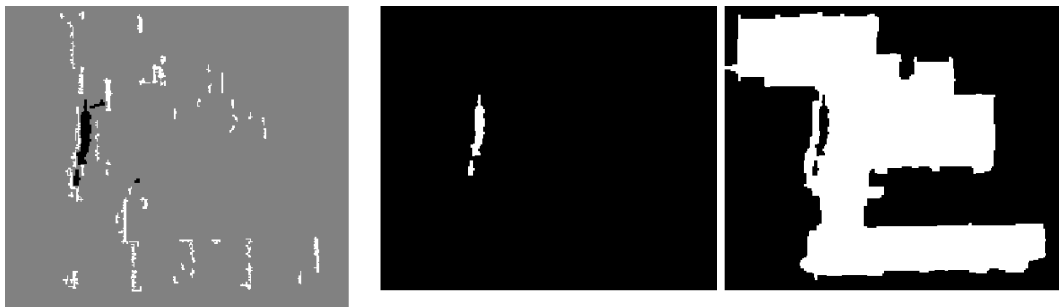
(g) Data gaps and facades together (h) Only data gaps adjacent to facades are selected (i) Final building mask, modified using selected data gaps
