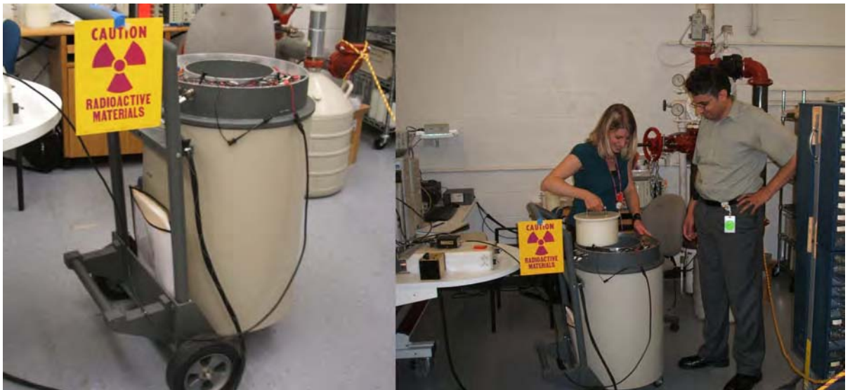
Figure 3.2: Left: JCC-51 AWCC on the test laboratory floor in the Meriden facility of Canberra Industries. Right: The author is shown removing the end plug with Dr Nabil Mena in attendance.
