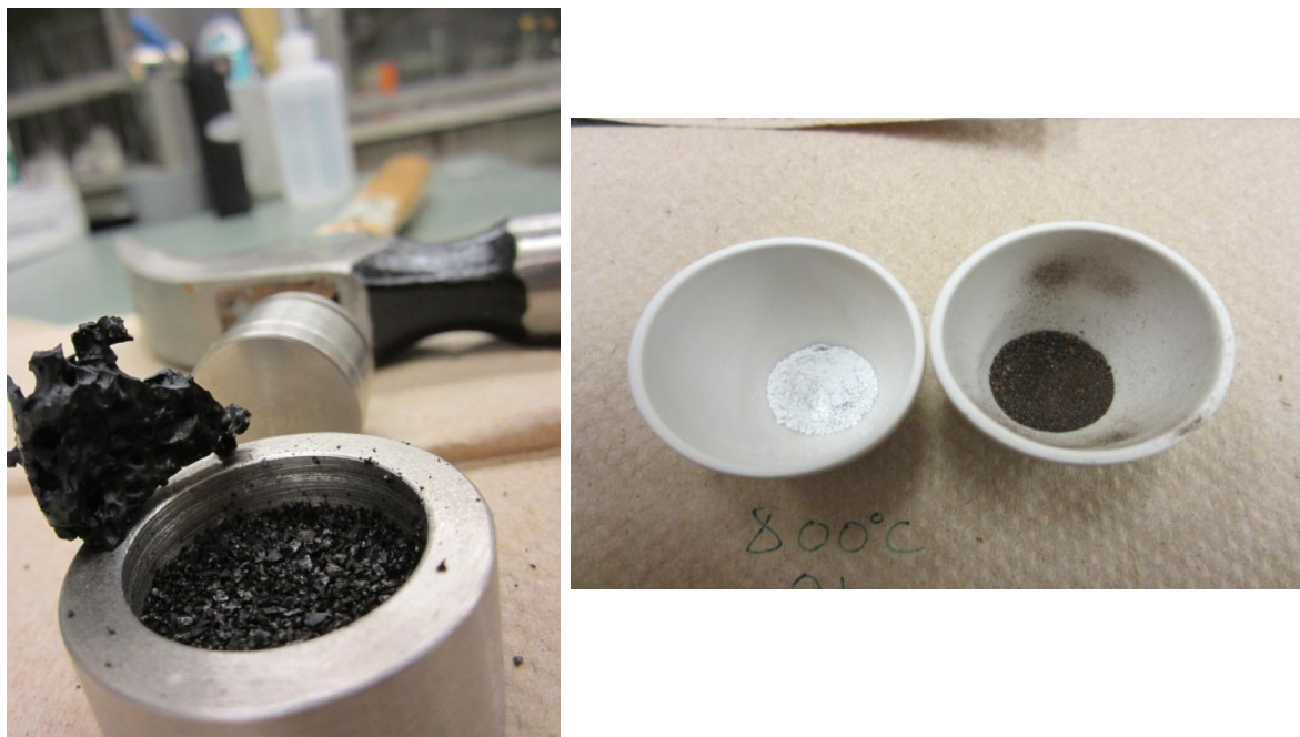
Figure 3.2 : (A) Aluminium container and lid used with a hammer to crush large pieces of decomposed pechini resin. (B) Transformation of the powder before (right) and after (left) thermal treatment.
