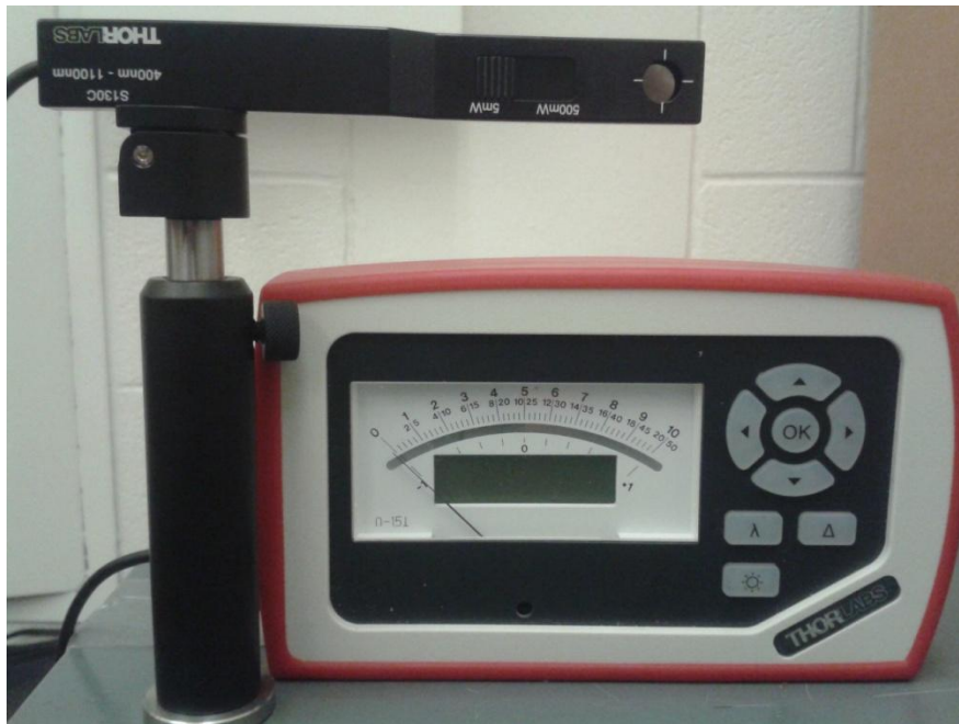
Figure 3.12 : Photometer ThorLab PM100 A, small receptor aperture (9.5 mm) with 2 degrees of sensitivity (5mW and 500mW). The luminescence measurements were done at the most sensitive level.
