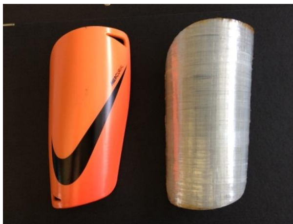
Figure 4.11 Football shin pad of Nike Mercurial (left) and the one made of SR-PLA composite (right).
