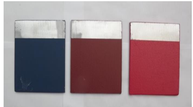
Figure 3 Laboratory plates before immersion (Left SPC, Middle CDP and Right AF)
