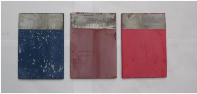
Figure 5 Laboratory plates after artificial immersion (Left SPC, Middle CDP and Right AF)
