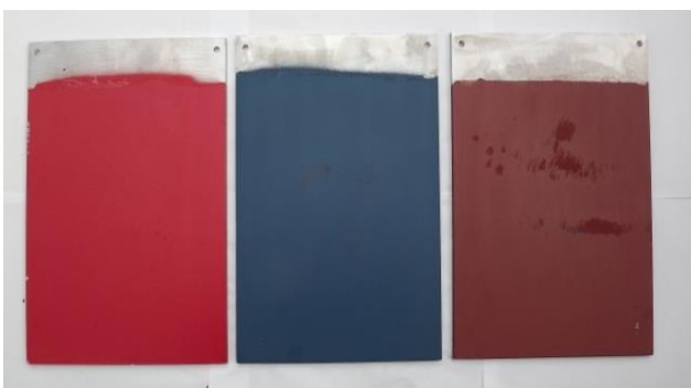
Figure 2 Sea Plates before immersion (Left AF, Middle SPC and Right CDP)
