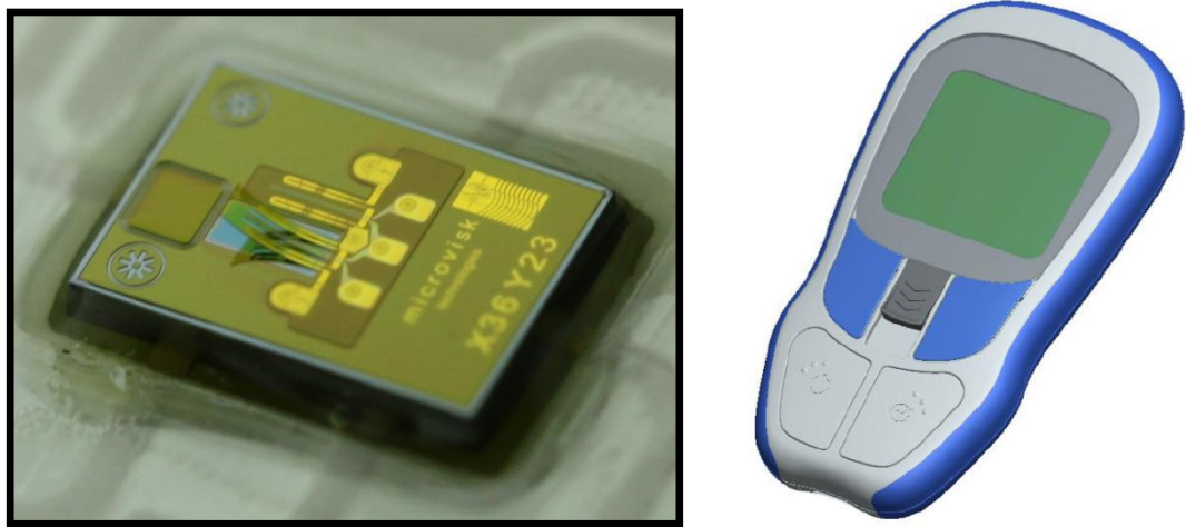
Figure 1.4: The MEMS sensor chip contained in each SmartStrip (left). The three-legged 'Epsilon design' of the released polymer microcantilever is visible protruding from the surface, with gold heater loops on the two outer legs and a constantan sensor in the centre. The reagent pad and contact vies are seen close to the tip and base of the beam respectively. The CoagMax handheld interface (right). Images courtesy of Microvisk Ltd.
