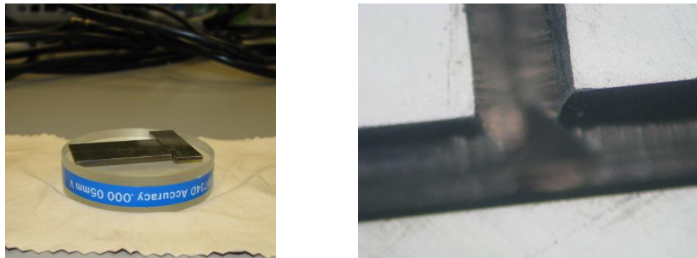
Figure 3.5 Metrology primary standards on an optical flat as used for the linearity calibration of the autofocus experiment (left). Example autofocus image for the standard trio showing the top right slab in focus (right).
