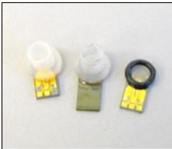
Figure 6.19 Three designs for containment of the silicone oils on the microcantilever sensor. Damaged chips were used to try out the different sample containment techniques. Left: sample fluidic well; Centre: Fluidic well mounted on top of an O-ring; Right: O-ring. It was found that the fluid well without the O-ring (left) was the best method as it incurred least losses in assembly.
