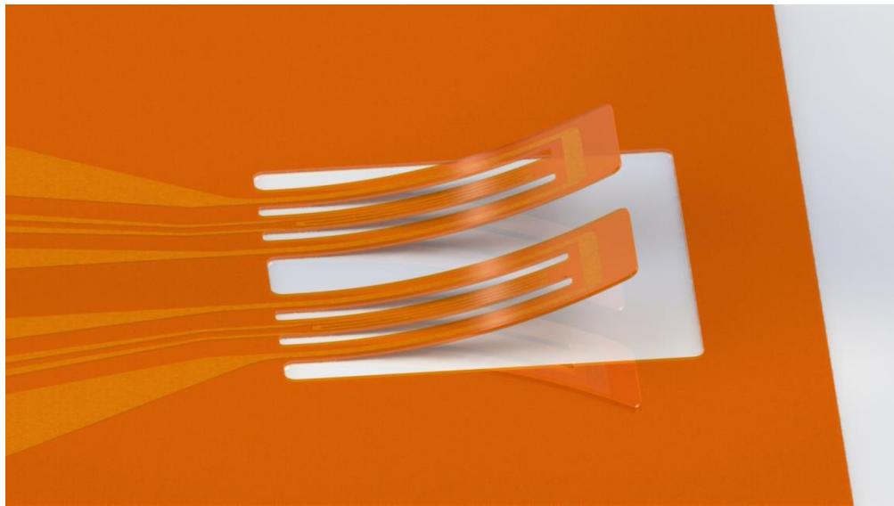
Figure 5.6 Schematic of Thermal Design (TD) microcantilever beam requirements. Outer dimensions are length = 750 \mu\text{m} ; width = 280 \mu\text{m} ; thickness less than 10 \mu\text{m} .
