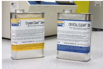
Figure 2.38: Part A and Part B of the polyurethane material
