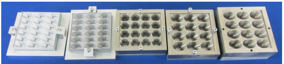
Figure 5.7: The five casting moulds used for the fabrication of the SEH concentrators (H1 to H3 - in order from left to right)
