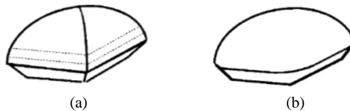
Figure 1.19: Design concept of a new three-dimensional (3-D) lens for a static concentrator: (a) previous 3-D lens; (b) new 3-D lens [74]
