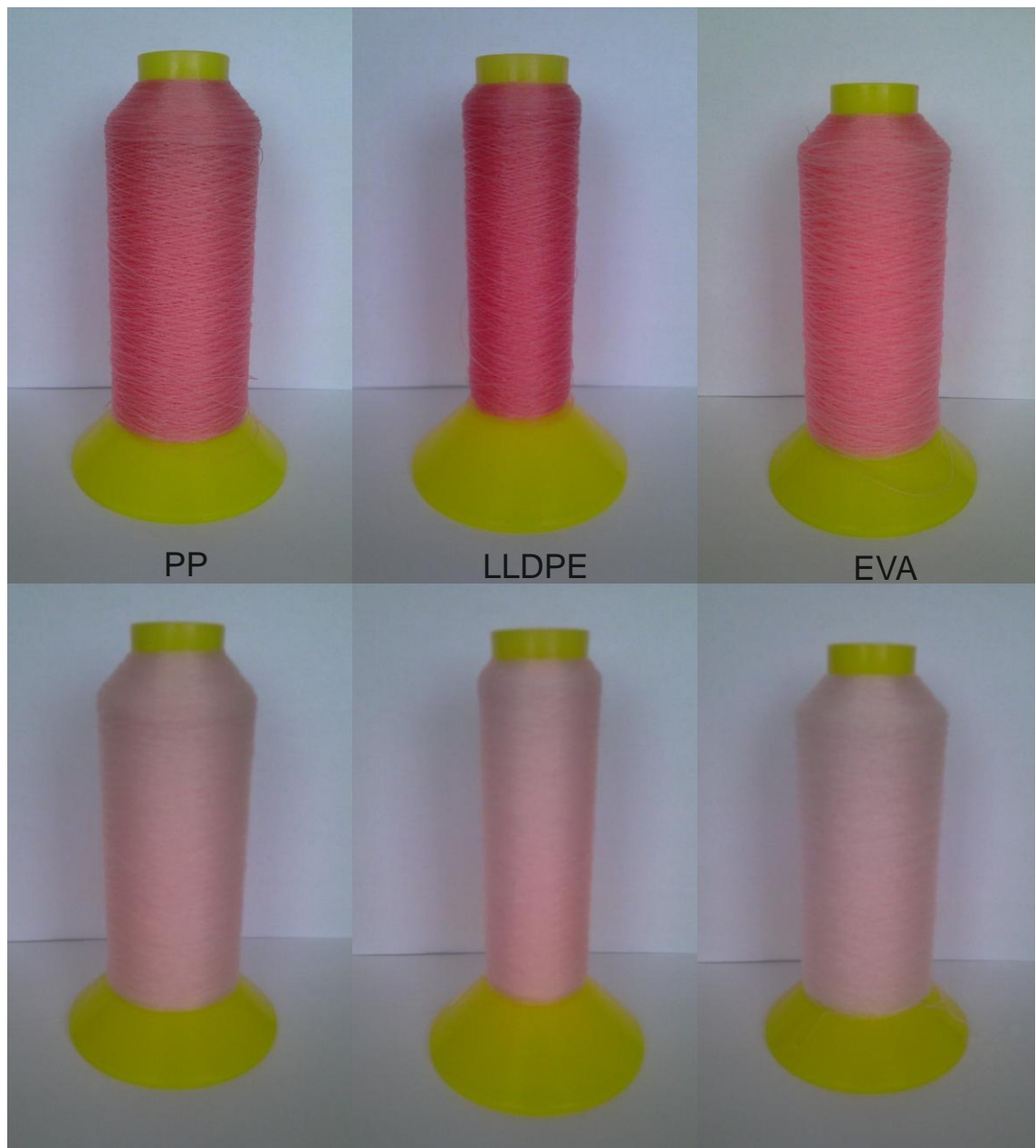
Figure 4.50 Thermochromism of polymers containing the red pigment
