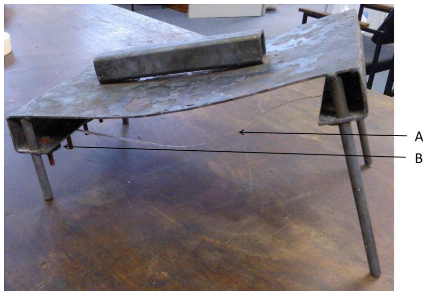
Figure 1 5 Bundles Steel Rig. A) GF Bundle. B) Nut, bolt and washer.
