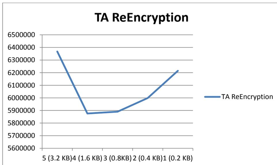
**Figure 33: Graph of data size against Re-Encryption time. X-axis showing data size in kilobytes, Y-axis showing time in milliseconds for re-encryption**
