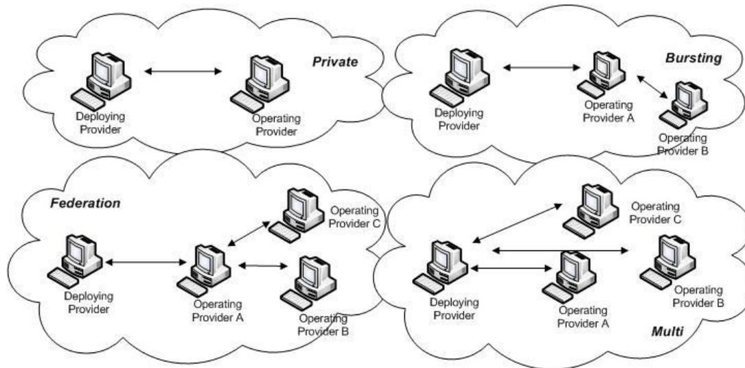
**Figure 7: Cloud Scenarios. (Private involves one deploying and one operating provider, Bursting - the operation provider can burst to another provider, Federation - a team of providers work together, Multi - the service can be deployed on a number of providers, acts as a broker)**
