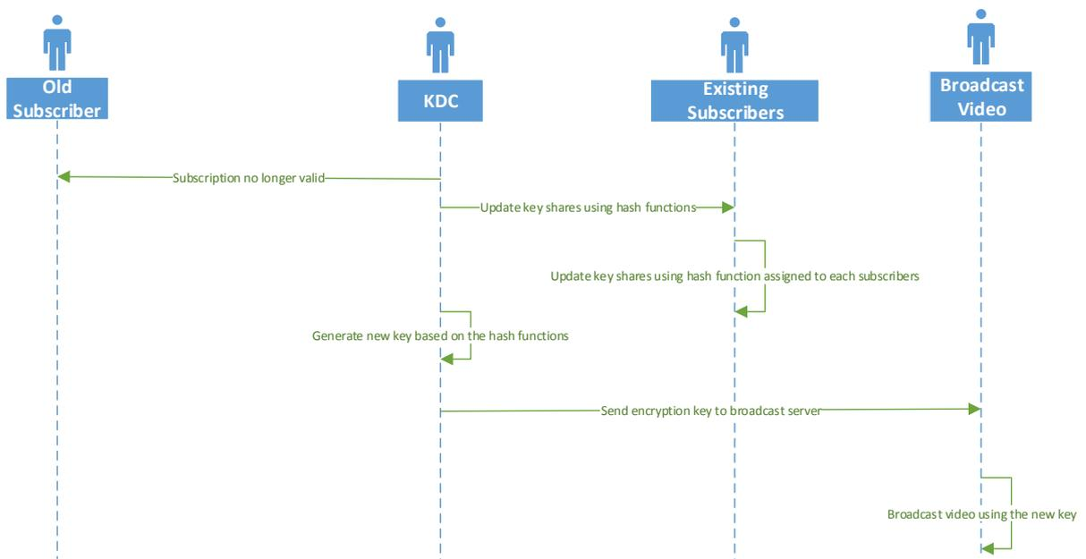
**Figure 19: Sequence diagram for user revocation and new key generation**
