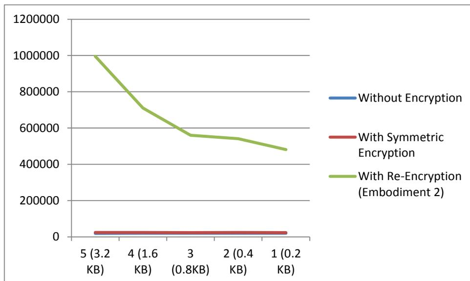
**Figure 32: Graph for different times recorded for the three scenarios. X-axis showing data size in kilobytes, Y-axis showing time in milliseconds for encryption**
