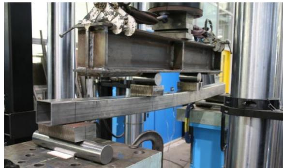
Fig. 8. Bending test set-up (4PB)
