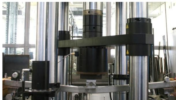
Fig. 9. Bending test set-up (3PB)
