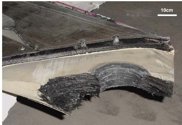
Fig. 12 Lug failure from the A300 Airbus tail from Flight AA589
