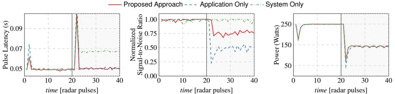
Figure 3: Radar results: performance, energy consumption and accuracy over time.
