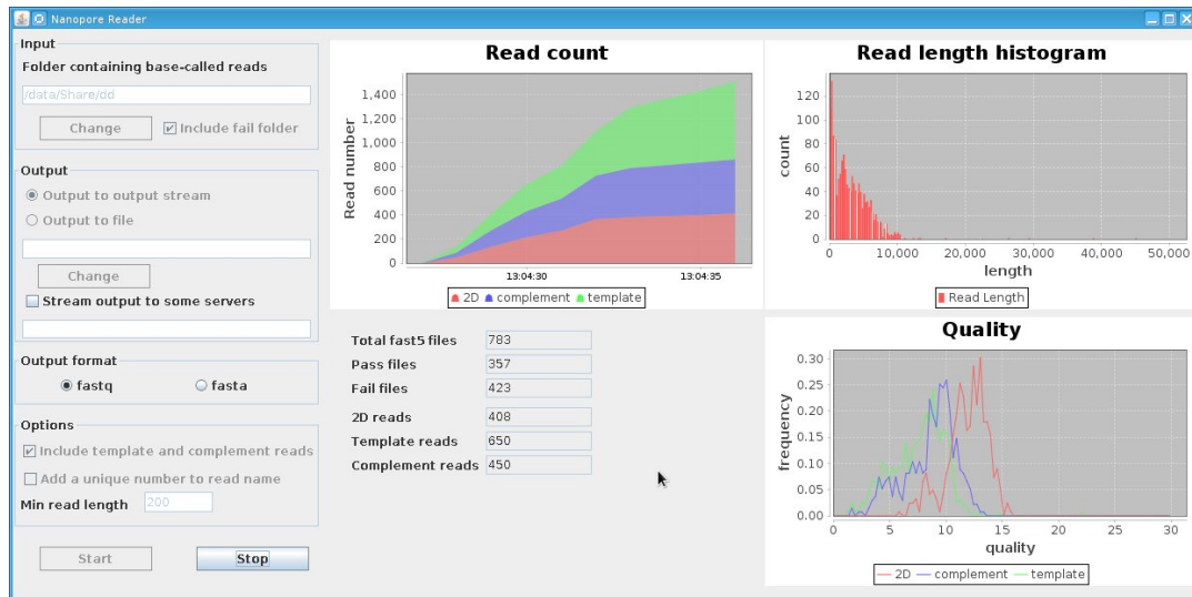
Fig. 1. A screen shot of npReader. User can specify options of data to be extracted and details of outputs in the left panel. The right panel displays statistics of data, including read counts, read length histogram and read quality in real-time.
