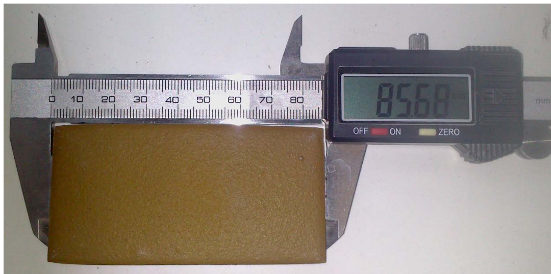
Figure A1. Photograph of sample produced with uncalcined 80 wt. % dry discharged fine IBA dust: 20 wt. % glass and sintered at 1080 °C
