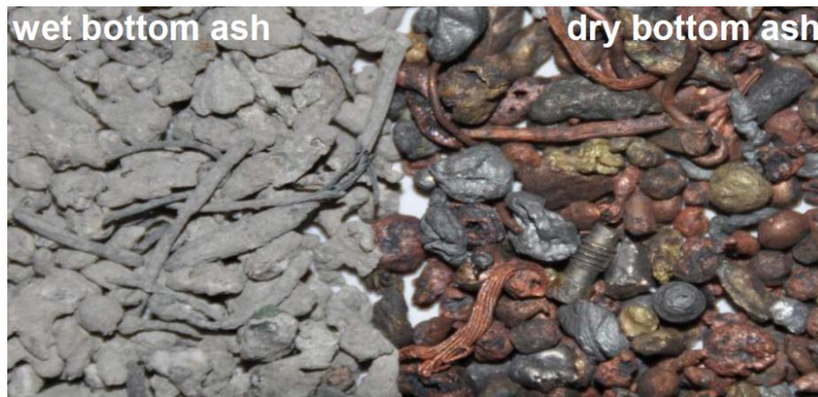
Figure 1.5: Difference between metals sorted from a wet and dry bottom ash. The discharge system of IBA has an effect on the degree of oxidation and the subsequent metal sorting process and performance (photos taken from ISWA-WGER).
