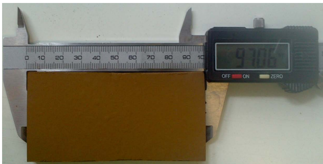
Figure A2. Photograph of sample produced with calcined at 1080 °C 80 wt. % dry discharged fine IBA dust: 20 wt. % glass and sintered at 1080 °C (optimum ceramic)
