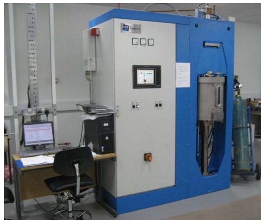
Figure 3.5 SPS facility at Queen Mary University London used in this work.
