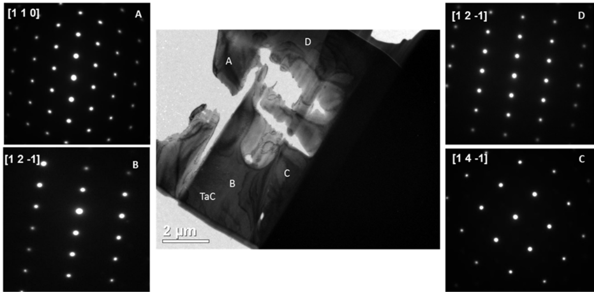
Figure 6.12 BF TEM image of FIB section of laser melted TaC and respective SAED indexed patterns showing cubic grains.
