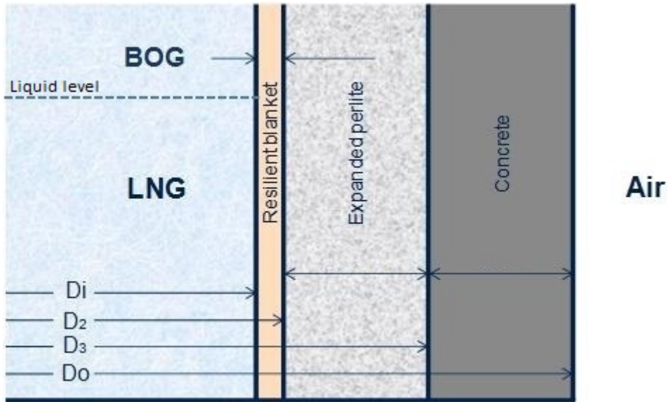
Figure 2 Above-ground LNG storage tank wall section
