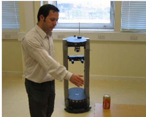
Fig. 3. The experimental setup involves an ActivMedia Peoplebot observing a human demonstrator acting on objects
