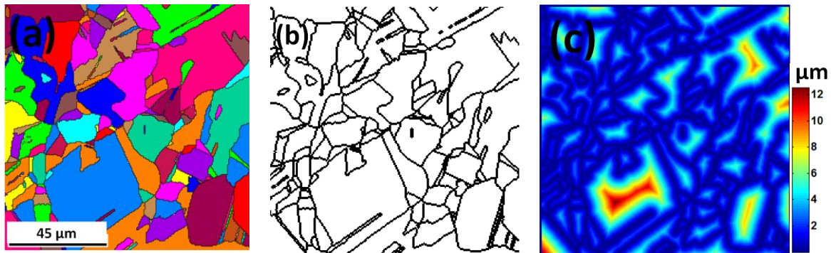
Figure 2, demonstration maps grain boundary and Euclidian distance calculations, using a map from Cu deformed to 10% strain, mapped over 112\mu\text{m}\times 112\mu\text{m} , 0.5\mu\text{m} step size (a) grain coloured map (b) binary grain boundary map. (c) Calculated shortest Euclidean distance to the nearest surface grain boundary.
