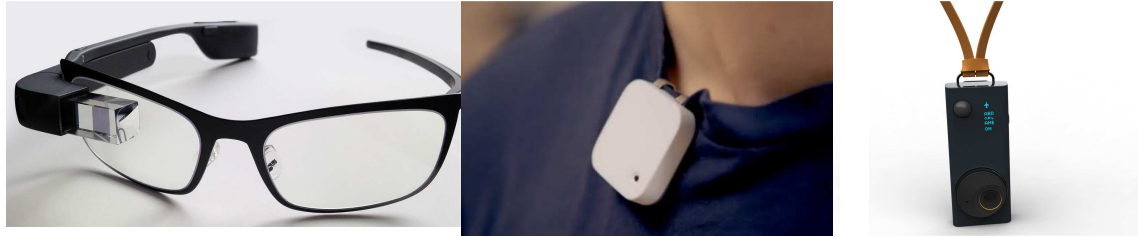
Figure 2.6: Wearable camera devices. From left to right: Google Glass, Narrative Clip and Autographer.
