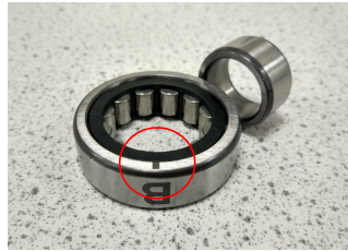
(b) Bearing B with outer race defect
