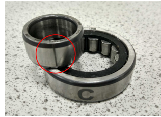
(c) Bearing C with inner race defect
