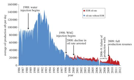
**Figure 9.** Daily oil production rate (average over a month) from the Ula field from start of production in 1983. WAG injection was started in 1998 and by 2000 it was clear that the decline in oil production had been stopped. Today almost all the oil production is believed to have come from EOR. The oil rate expected without EOR was estimated using numerical simulation. (Online version in colour.)
