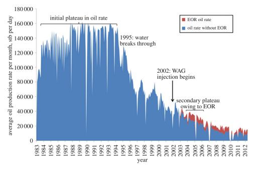
**Figure 8.** Daily oil production rate (average over a month) from the Magnus field from the start of production in 1983. WAG injection was started in 2002 and by 2005 it was clear that the decline in oil production had been reduced. The oil rate expected without EOR was estimated using numerical simulation. stb, stock tank barrel. (Online version in colour.)
