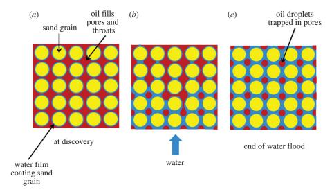
**Figure 3.** Illustration of oil trapping in a water-wet rock. (*a*) At discovery the sand grains are coated with a thin water film and the pores are filled with oil; (*b*) as water flooding progresses the water films become thicker until (*c*) the water films join and oil continuity is lost.
