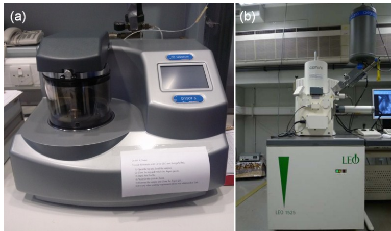
Figure 4.14: (a) Chromium sputter coating machine and (b) FEG-SEM
