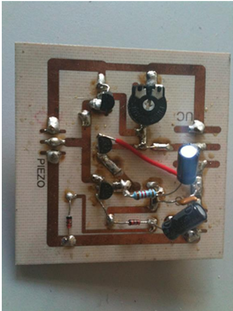
Figure 29: Actual PCB implemented transmitter PZT disc driver
