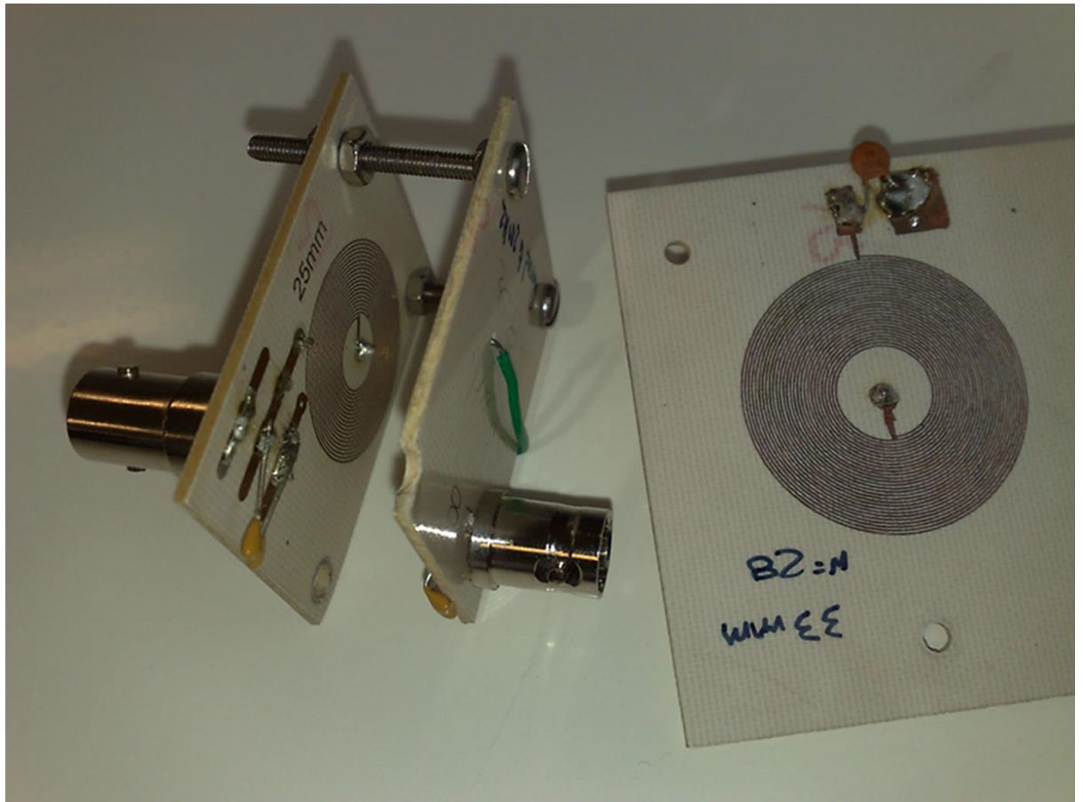
Figure 38: Fabricated printed spiral coils on PCB
