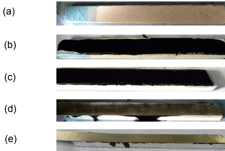
Figure 2. Stages in the manufacture of the peel specimen, (a) preparation of the aggregate, (b) applying the pre-heated bitumen onto the aggregate, (c) placing the wire spacers, (d) placing the peel arm on the top and (e) a ready-to-test specimen.
