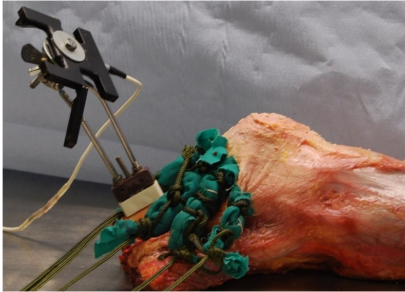
Figure 4.19 The tracker used to record femoral motion fixed with a custom made mount to the femur.
