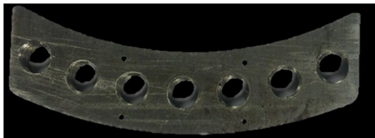
Figure 7.26 The second plate developed for fixation to the anterior tibia. The central hole is to correspond to the anatomical TT position and the holes to the right and left sides to permit progressive 5mm medialisation and lateralisation up to 15mm. The small holes in the top and bottom rows of the plate were used to fix K-wires through as an alternative to the screws planned for use in the first image.
