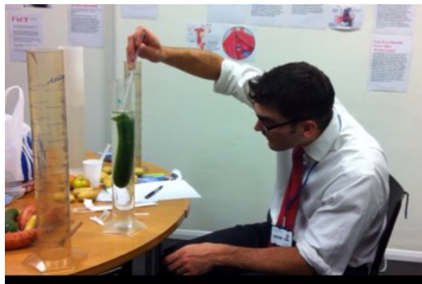
Figure 18: Volume estimation using displacement method
