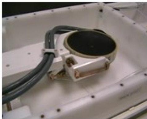
Figure 43: Five axis robotic transducers
