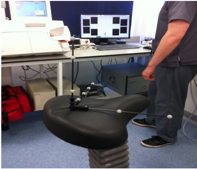
Figure 5.2: Step 1 of the OEP system calibration using the Reference Frame Assembly tool.
