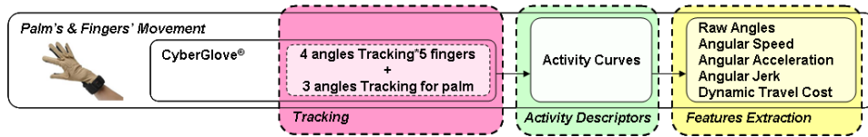
Figure 4.16.: Flow Chart diagram of the procedure followed for the extraction of dynamic features from the movement of the fingers.
