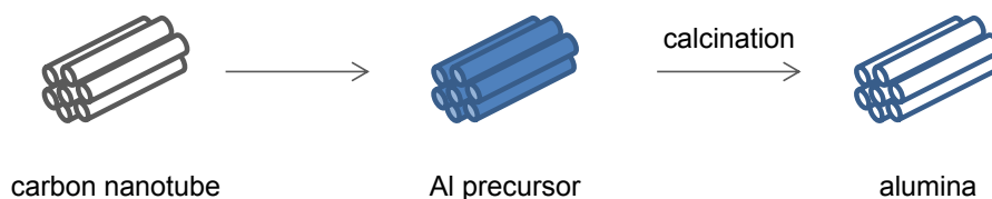
Figure 4.1. Schematic pathway for organised mesoporous alumina synthesis.
