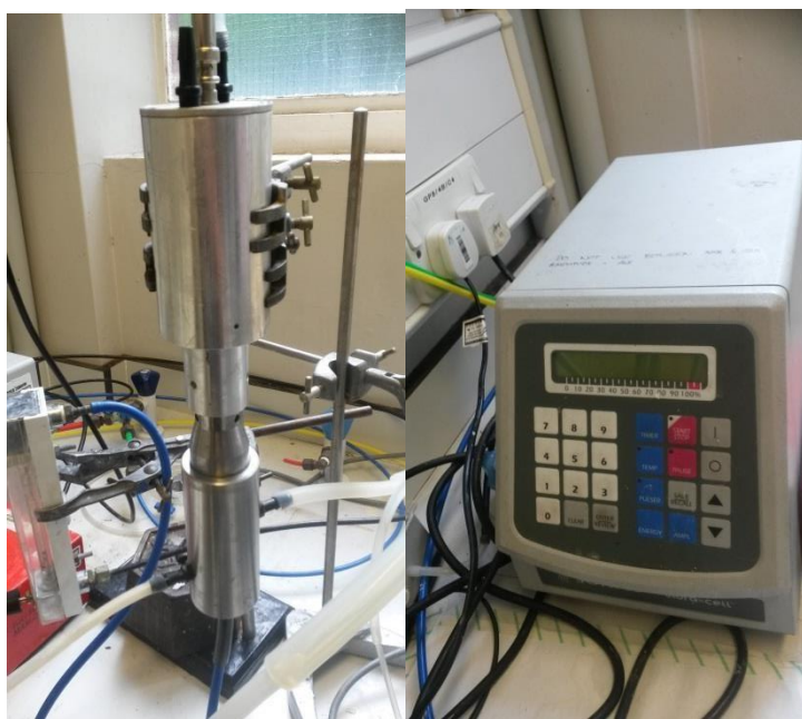
Figure 3-1. Picture of the Sonication probe and flow through cell (left image) and the base unit for the sonication probe (right image).
