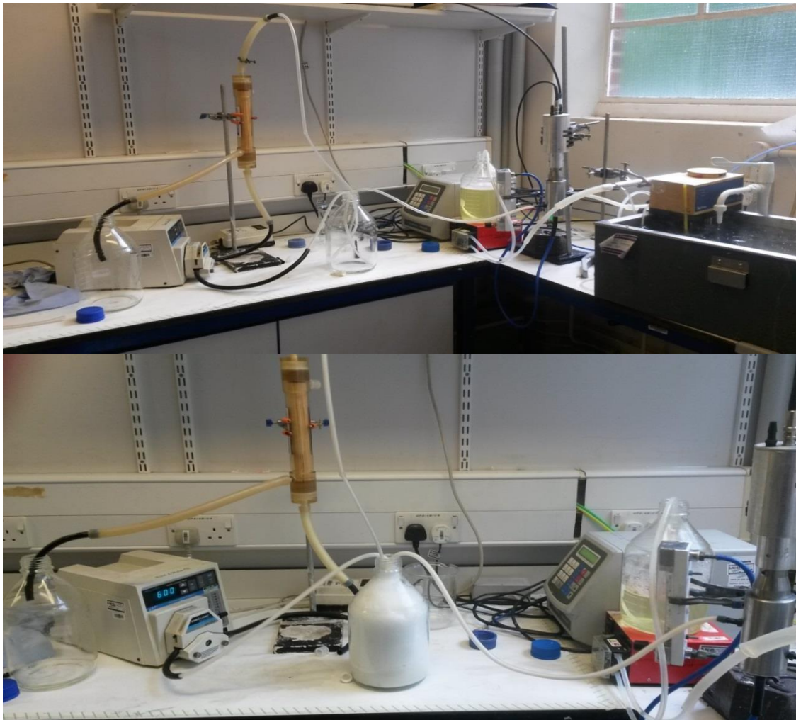
Figure 6-4 Images of the cross flow filtration one stage process. Top Image= Before the experiment started, Bottom Image= During the experiment.
