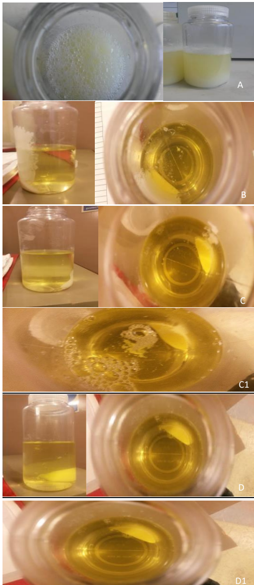
Figure 3-7. A series of images showing the progression of the centrifuge step. A= 0 minutes, B= 20 minutes, C=40 minutes, C1=40 minutes after slight agitation to the vessel, D=60 minutes, D1= 60 minutes after vigorous agitation to the vessel.
