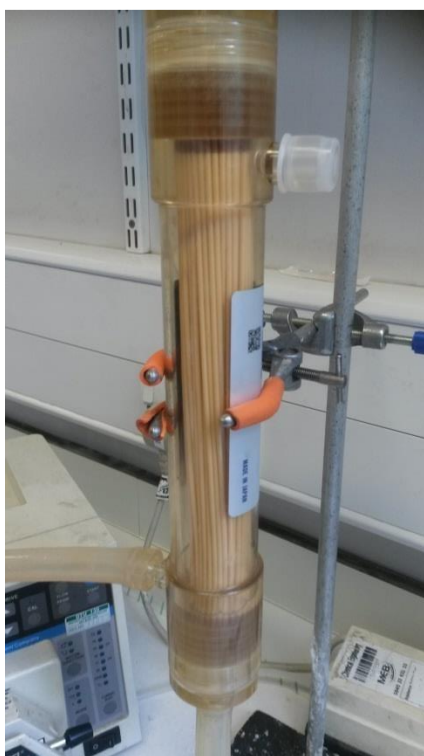
Figure 6-1. An image of the cross-flow filtration module used during the experiments.
