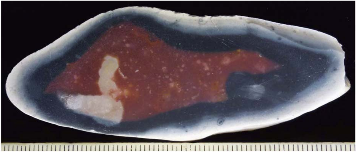
Text-fig. 18. Red flint from the Turonian Chalk of Helgoland. The well-defined red zone in the centre of the core is surrounded by black flint, and then by a white cortex
