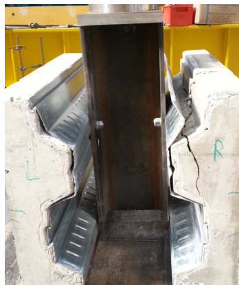
Figure 10. Deck de-bonding in left slab and rib shear failure in right slab of specimen M2
