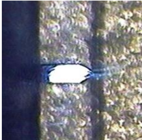
Figure 2: AFM cantilever aligned above the central aspect of a PPTA fibre
