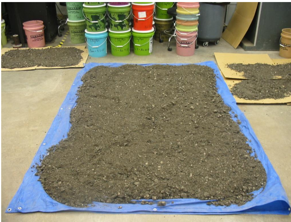
Figure 5-1. Drying process of RAP materials in the laboratory
