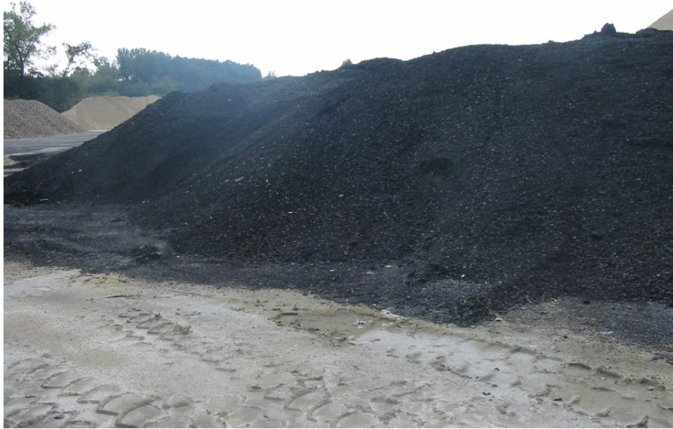
(a) RAP stockpile
