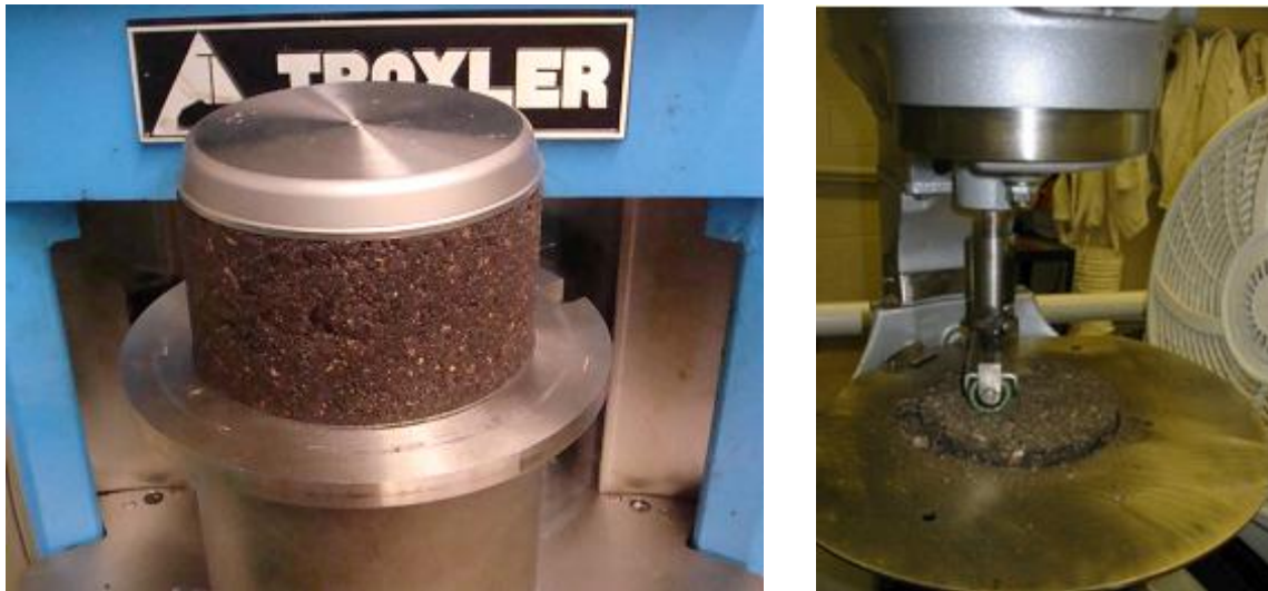
Figure 8-22. Pictures of raveling testing specimens and equipment
