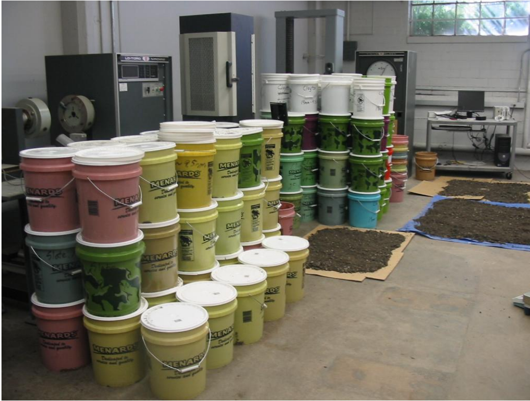
Figure 5-2. Sorted RAP materials in 5-gallon buckets
