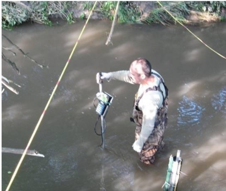
Figure 12. FlowTracker. Velocity measurements using a FlowTracker are needed to develop a stage-discharge rating curve.
