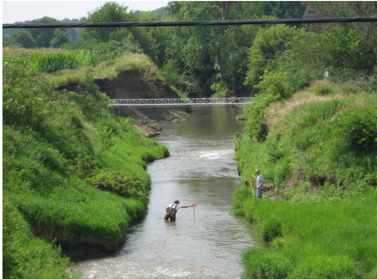
Figure 14. Survey of the knickpoint. Bi-annual surveys of the channel morphology were conducted at the knickpoint study site.
