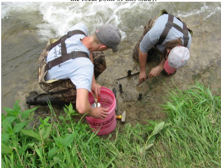
Figure 10. Bed and Bank Sampling. Samples of the stream bed and channel banks were collected for geotechnical analysis.
