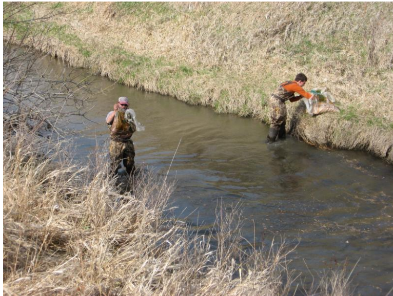
Figure 13. LSPIV. (a) The LSPIV truck collects video imagery of seeded particles in the stream to determine the free surface velocity. (b) Seeding of the stream with eco-safe mulch for LSPIV measurements.
