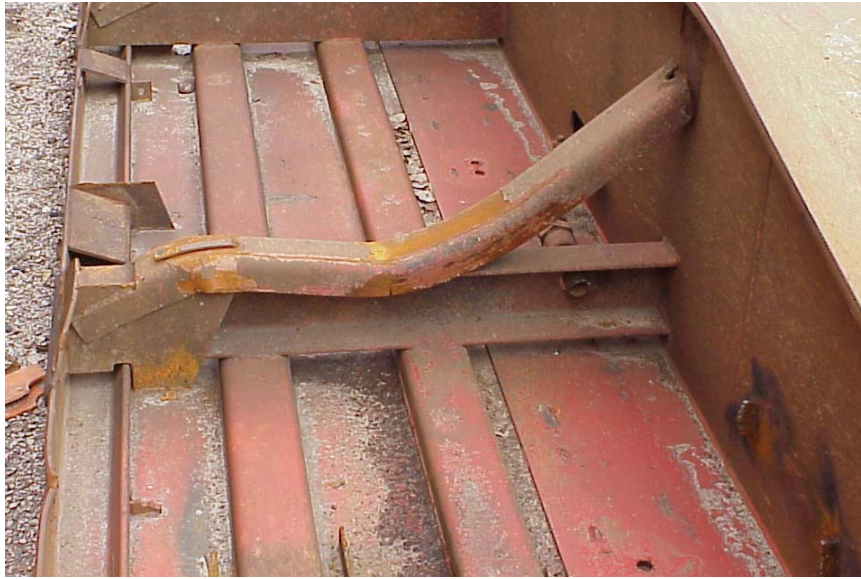
Figure 2.8. The deformed transverse member in AF4.
