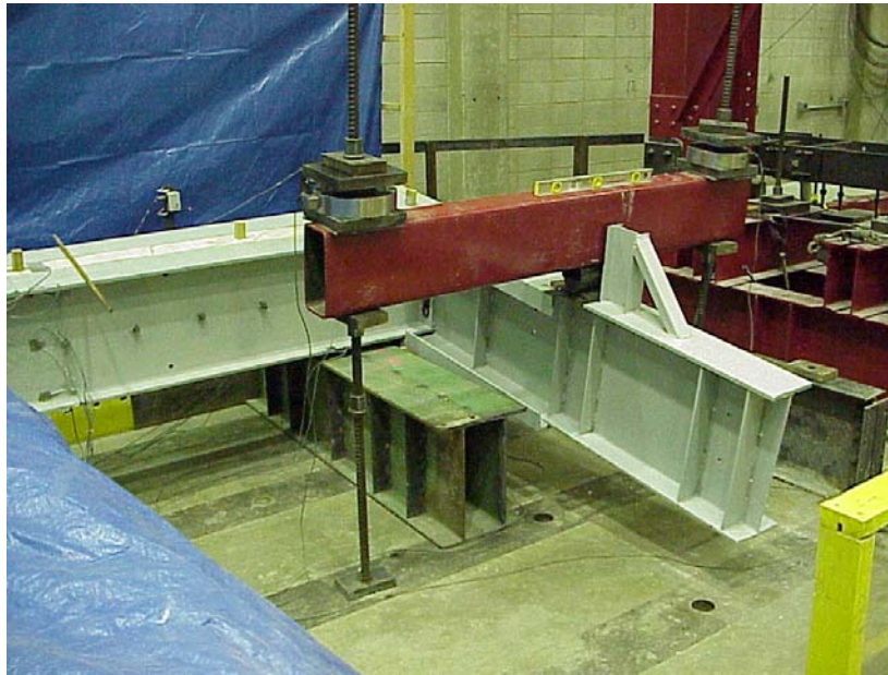
a. Loading system and lever arm rotation
