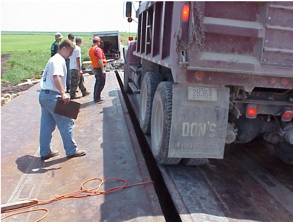
Figure 4.17. North eccentric transverse position of the truck in BCB LT1.
