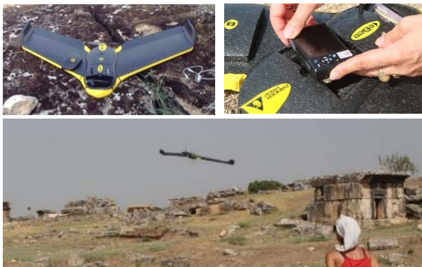
Figure 1: The setting up of the fixed wing eBee platform with the customized camera and take-off phase.
