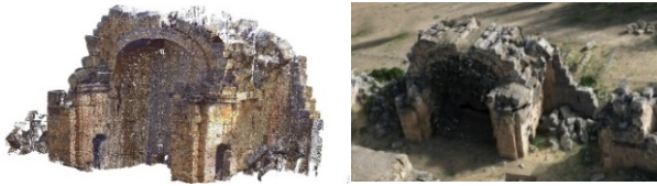
Figure 3: The entire complex and corresponding views of LiDAR model and the drone one, quite deficient in upstanding walls, especially high.
