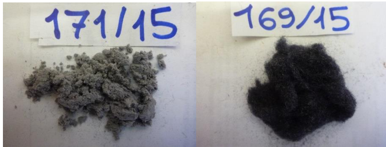
Figure 50: Ambiance (171/15) and machinery sampling (169/15) from weaving section.
