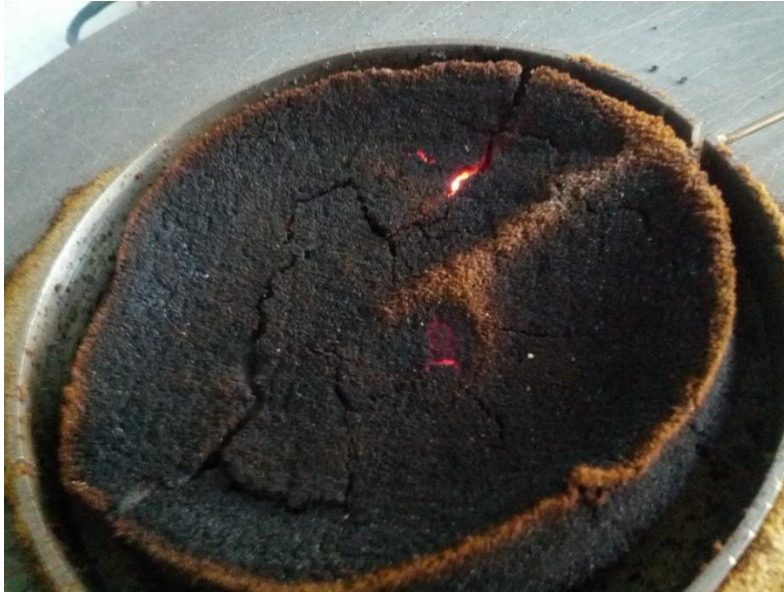
Figure 10: Evidence of ignition in the hot plate standard test for LIT, glowing combustion within the dust layer sample.
