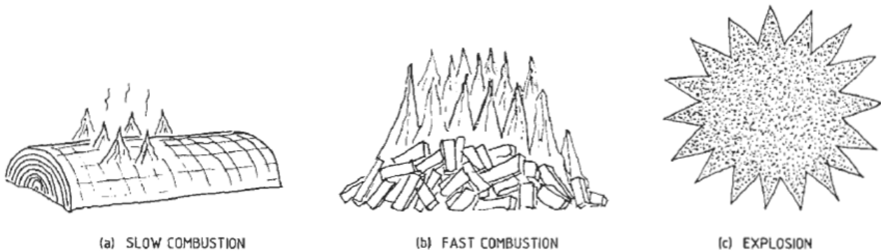
Figure 4: Schematic drawing that shows the influence of particle size with respect to combustion kinetics, from Echhoff (2003).
