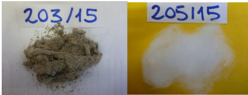
Figure 48: Carding section samples, from ambiance (203/15) and machinery sampling (205/15)
