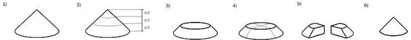
Figure 7: Schematic representation of coning-quartering sampling method
