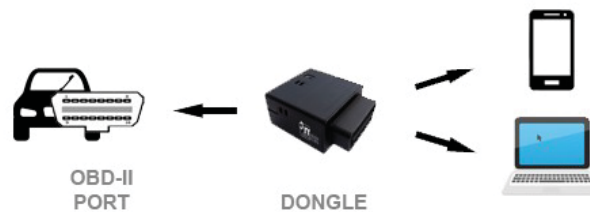
Fig. 9. A dongle can be connected to the OBD-II port to allow brought-in devices to access vehicle data.
