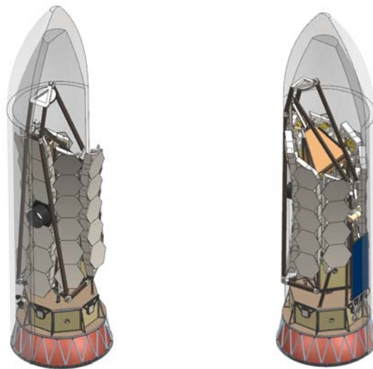
Figures 7 and 8 - ATLAST 9.2m Primary Mirror in a 5 m Fairing
