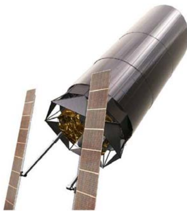
Figure 3. ATLAST design concept utilizing an 8 m monolithic primary mirror.
