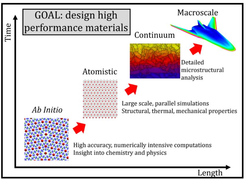
Multiscale modeling breaks down the elements of material design factors to their relevant time and length scales. The chemistry of a material can be probed with quantum mechanics; its thermal and mechanical properties, with atomistic techniques; and its micro- and macro-scale properties, with continuum methods. As shown in the chart, the output of one level is passed on to the next level, creating a powerful predictive model. John Lawson, Alexander Thompson, NASA/Ames
