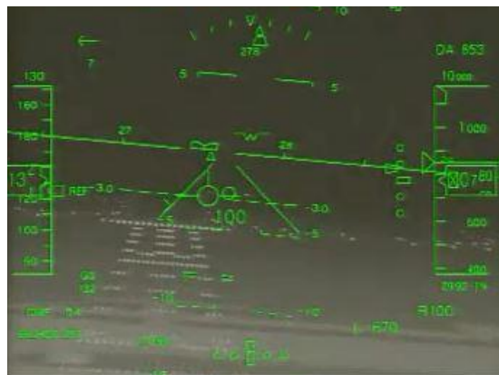
Figure 1. EFVS HUD with edge lines and guidance cue referenced to offset localizer navaid.
